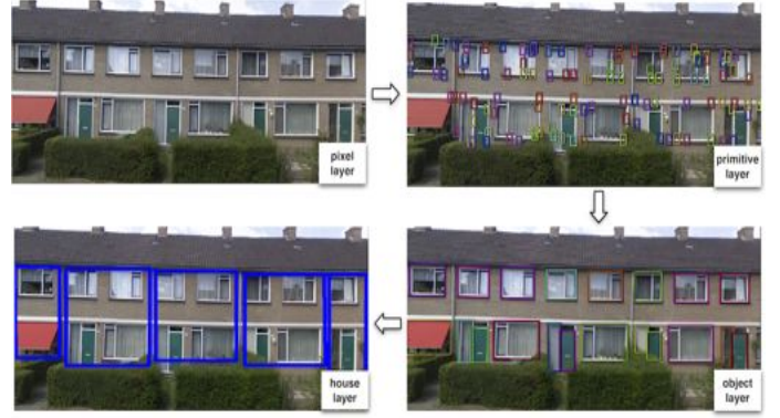
Figure 6: Data flow in the four-layer hierarchy of the facades domain. Input layers: pixels, corner primitives and object entities. Corresponding output layers: corner primitives, object entities and house entities, respectively.
